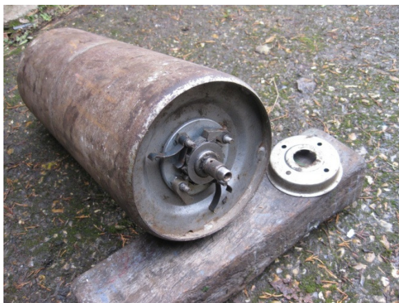
The rear-roller mechanism is stripped down, lubricated and reassembled with new components (such as bushes and springs)
