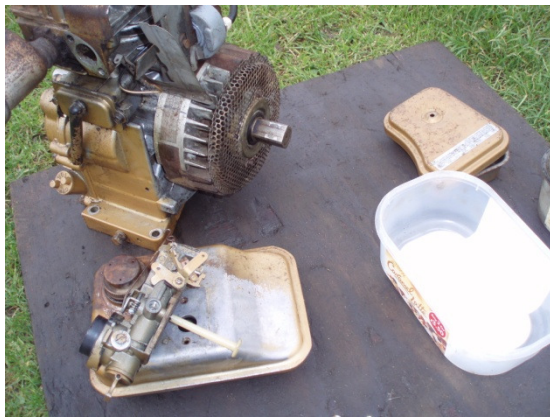
We rebuild the Briggs & Stratton engines' carburettors and recondition them internally by replacing pistons and re-seating valves
