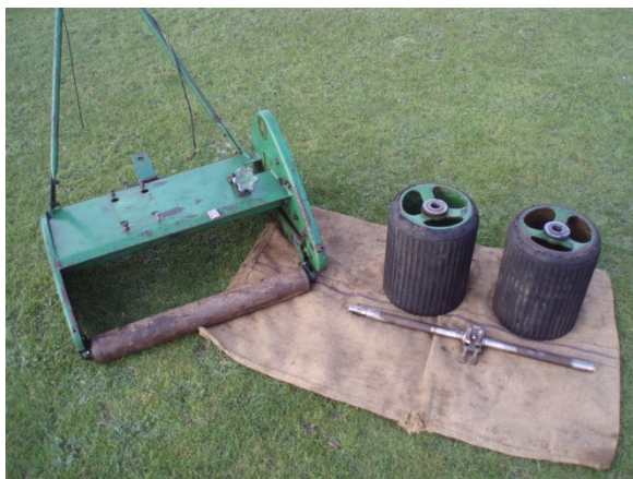
The rear-roller assembly removed from a Matador awaiting lubrication of the differential and reassembly
