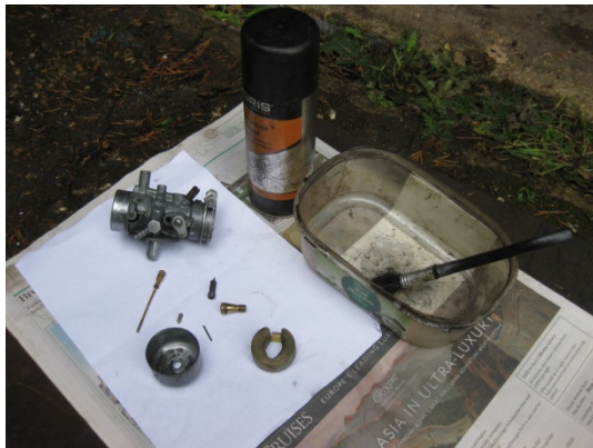
The MAG engine's carburettor and pull-start stripped down to be overhauled
