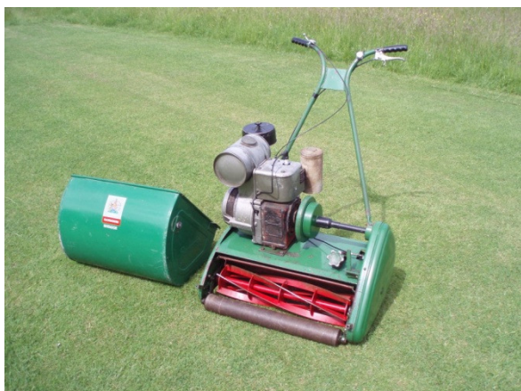
A reconditioned Ransomes Matador with its MAG 1026 engine having been rebuilt
