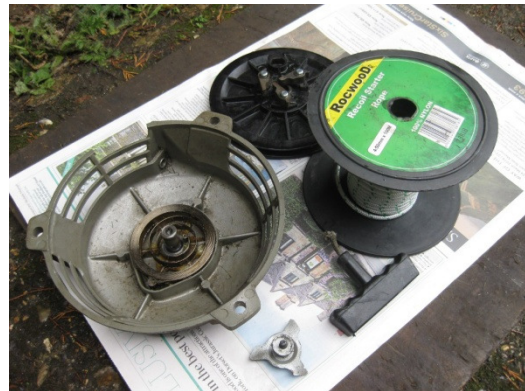
The MAG engine's carburettor and pull-start stripped down to be overhauled
