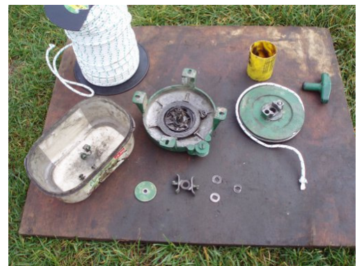
Carburettor, Ignition and pull-start overhauled (inspected/ tested and new components fitted)
