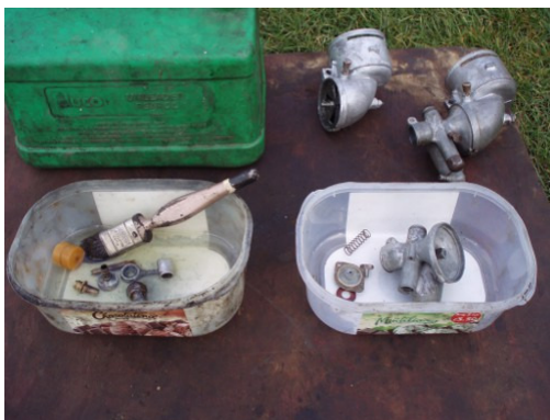
Carburettor, Ignition and pull-start overhauled (inspected/ tested and new components fitted)
