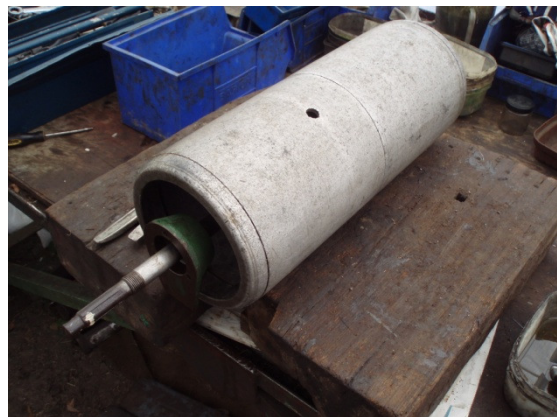
Auto-Certes Rear-Roller Differential lubricated- reconditioned and reassembled
