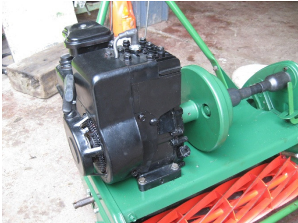
The Auto-Certes Mark 3M's original Briggs & Stratton engine- reconditioned to align with and operate the mower's clutch correctly
