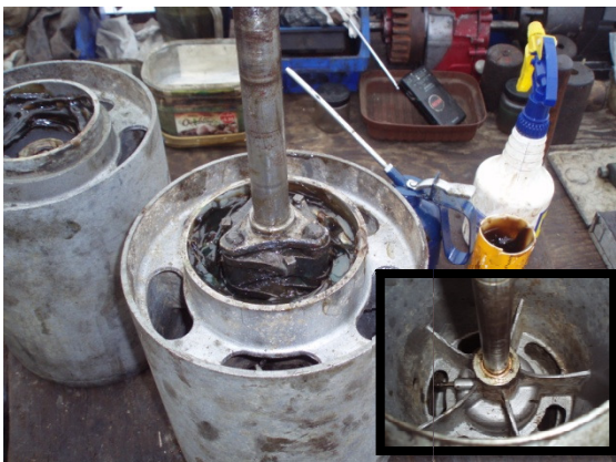
Auto-Certes Rear-Roller Differential lubricated- reconditioned and reassembled
