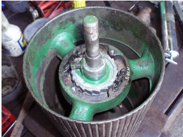
The Ajax Rear-Roller/differential mechanism (with the aluminium bevel gear in its centre). Our reconditioned Ajaxes are fitted with the best quality unworn components
