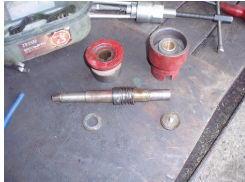
Photos showing the Light-Atco's clutch stripped down and ready to be overhauled
