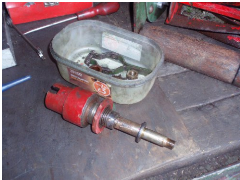
Photos showing the Light-Atco's clutch stripped down and ready to be overhauled
