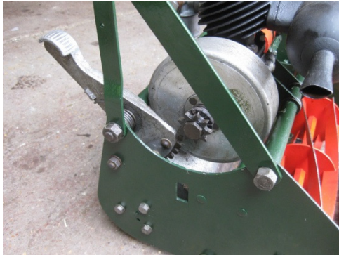
The condition of the pedal, sprocket/ratchet and spring is key to smooth operation
