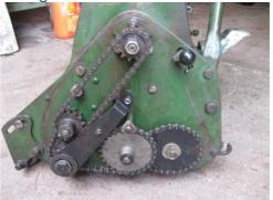
The Webb 24 (left) and Atco Royale (right) chain mechanisms are strong and well made but need to be adjusted regularly and/or replaced when they reach a certain level of wear
