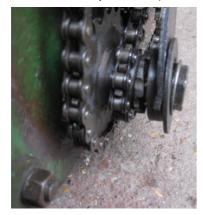
We fit new and unworn ratchet/sprockets, which will last for many decades with basic maintenance
