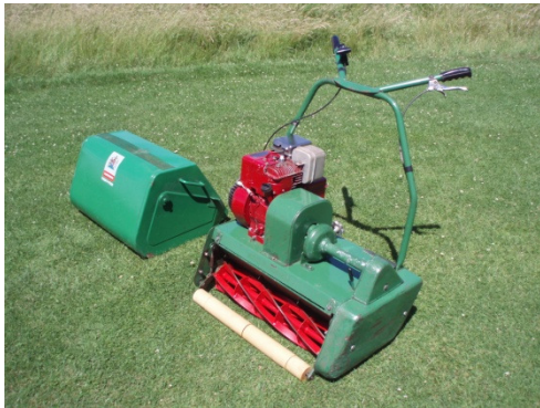
Reconditioned Ransomes Twenty-Four with new wooden front rollers
