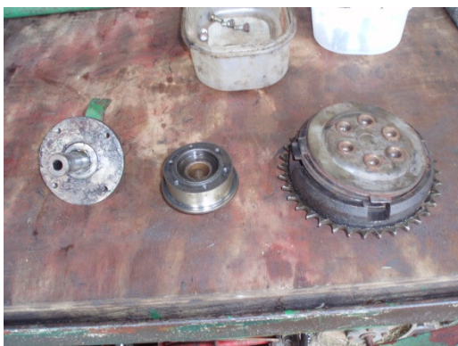
Rear-Rollers on Twenty-Four, with differential gears in their centre
