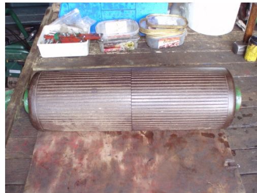
Rear-Rollers on Twenty-Four, with differential gears in their centre
