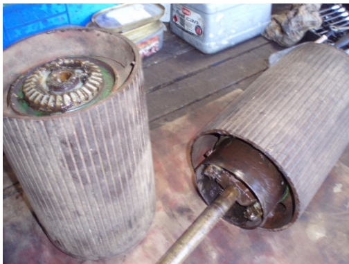
Rear-Rollers on Twenty-Four, with differential gears in their centre
