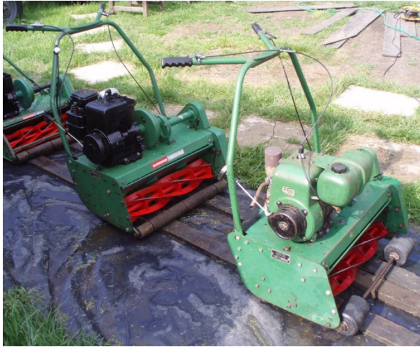
Two Ransomes Twenty-Fours with Briggs & Stratton engine (left) and Villiers F15 (right)- both mowers and their engines have been rebuilt
